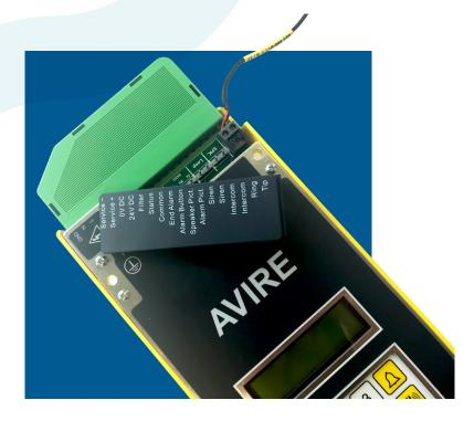
The Memcom+ emergency telephone provides both a fully compliant EN81-28 & EN81-70 autodialler and an engineers intercom for safer and more efficient installations. Memcom+ connects to our 'Multi Point Station' (MPS) accessories by a simple two-wire bus. The MPS units, powered and battery backed by the Memcom+, act as both engineer intercom points and EN81-28 remote alarm points.
